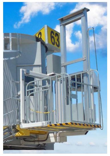
The Baggage Lift is a bridge mounted wheelchair and luggage lift that is capable of moving loads up to 500 lbs. from the bridge to the ground. It is not certified for lifting live loads, nor humans or pets. The Nova Baggage Lift has been approved for installation on JBT and ThyssenKrupp Passenger Boarding Bridges.
