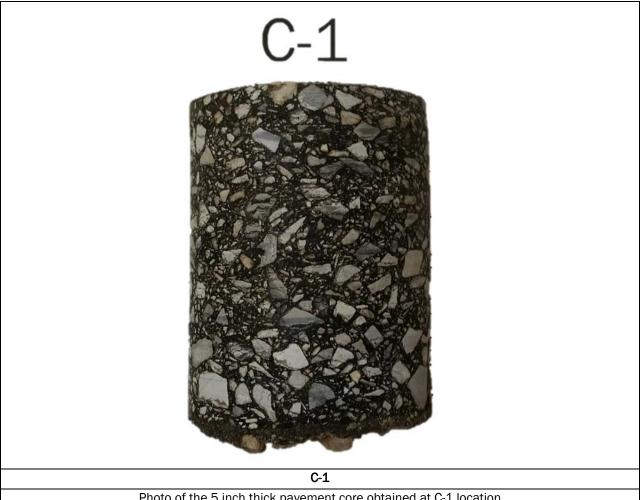
Photo of the 5 inch thick pavement core obtained at C-1 location
